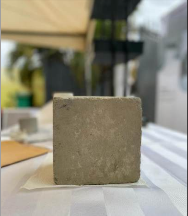
A sample of zero-cement geopolymer, above, a full-scale prototype made using geopolymer blocks, top right, and Evans Nartey, Theseus cofounder, bottom right.
