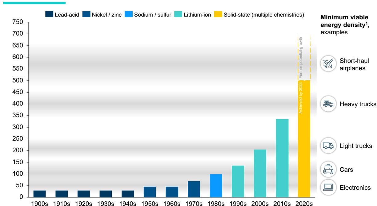
1. Minimum density at which first full battery-electric models are feasible
