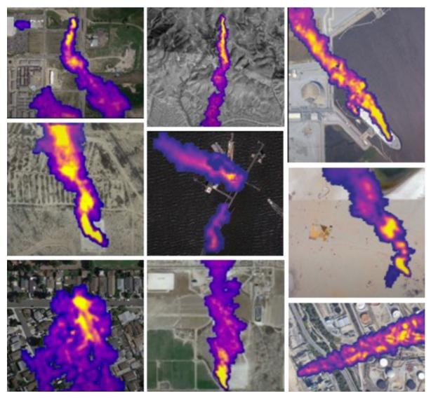
Note: Yellow plumes represent the highest methane emissions measurement. Image identification from left to right, top row: oil well unloading, gas storage tank, and LNG tanker; middle row: unlit flare, offshore platform, and gas compressor station; bottom row: gas pipeline leak, unlit flare, and chemical plant.
