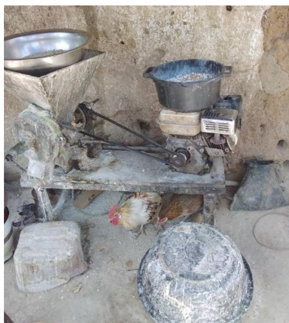
Ayuba Tasiu's 5.5 horsepower petrol grinder for wet milling cowpeas in Anguwan Malam Dogo, Kaduna state. Mr. Tasiu uses the same mill for making soybean flour.
