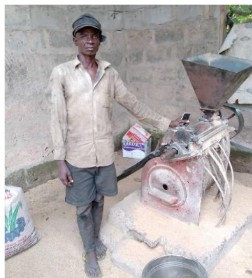
Otala Ibe is a rice miller in Cross River state. His old, single-stage mill removes rice bran but also breaks a large fraction of the kernel in the process. Replacing mills like his with electric, two-stage mills is rated “deployment-ready” for all criteria.
