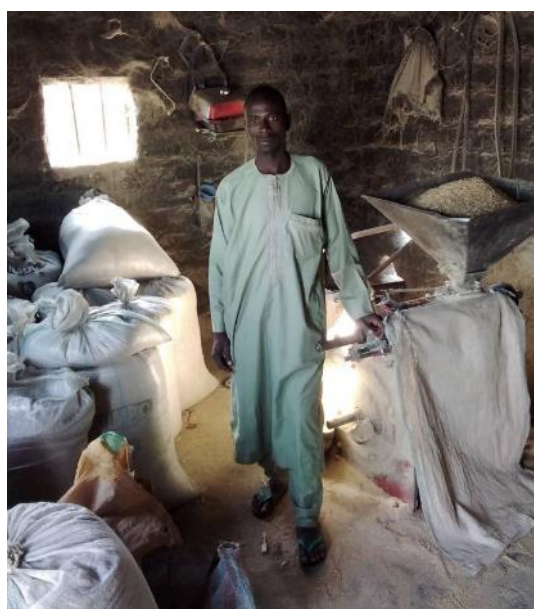
Habibu Lawal with his 25 hp diesel one-stage rice mill in Zagezagi community, Kaduna state. Habibu reports spending N4600 on diesel alone during a busy day of milling, and an addition N5000 per month for maintenance of the aging motor. This mill yields 50 kg of milled rice for every 100 kg bag of paddy rice. New mills can improve quality and boost milling yields by 20–30%.
