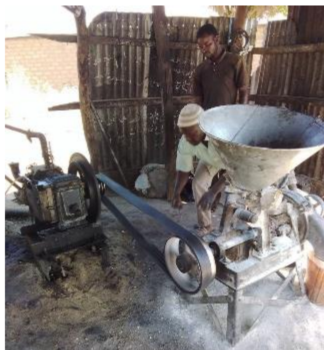
Ishaq Haruna running his 22 horsepower diesel flour mill in Kadage, Kaduna state. Mr. Haruna spends $4.40 US per day on diesel to run his mill compared to an estimated $1.80 he'd spend on electricity from a mini-grid with a $0.60/kWh tariff.
