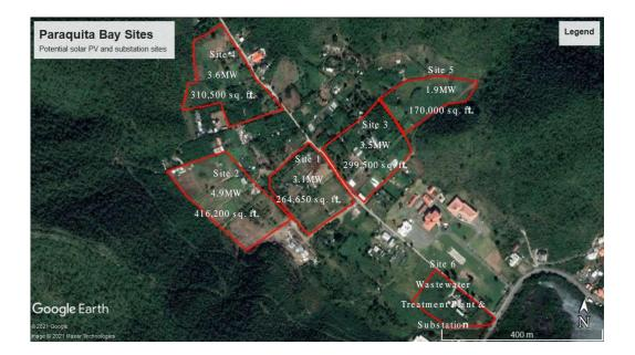
Sites 1-5 will be used for the ground mount solar arrays. The grounds of the wastewater treatment plant (Site 6) will be used for the substation.
