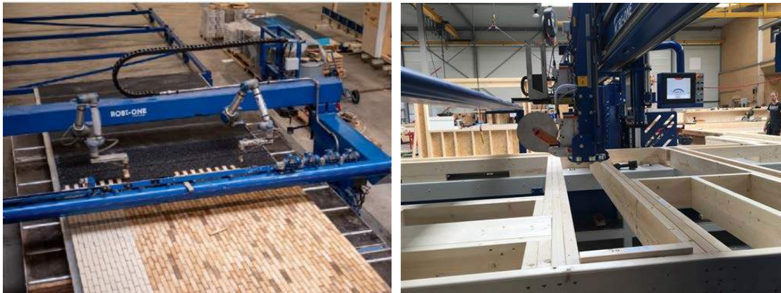
Figure 5. Timber frame manufactured with robotic exterior cladding application (left) and CNC machine (right)
