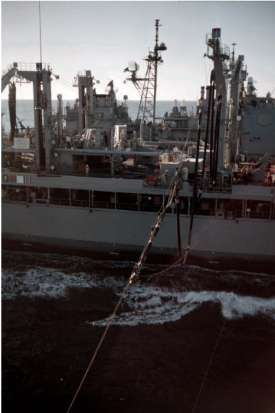
CG-59 pulls over a fuel line from an oiler. A single complete filling of CG-59's tanks would incur a delivered cost of about $0.85 million. CG-59 uses approximately $5.8 million worth of delivered fuel in a typical year, and is more efficient than three-fourths of the Navy's 27 hulls of this class. Chris Lotspeich photo.
