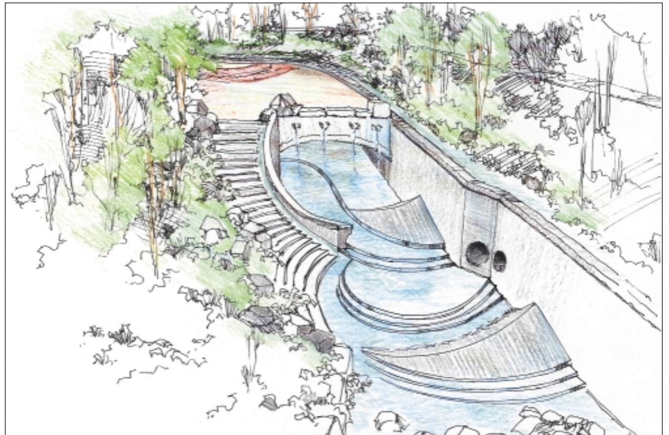
The outfall of the main Nine Mile Run culvert into the open channel at Regent Square Gateway. Smaller culverts emerge from the side walls. The sculptural structures in the channel celebrate the emergence of the stream and dissipate storm flow energy. Drawing by charrette team.
