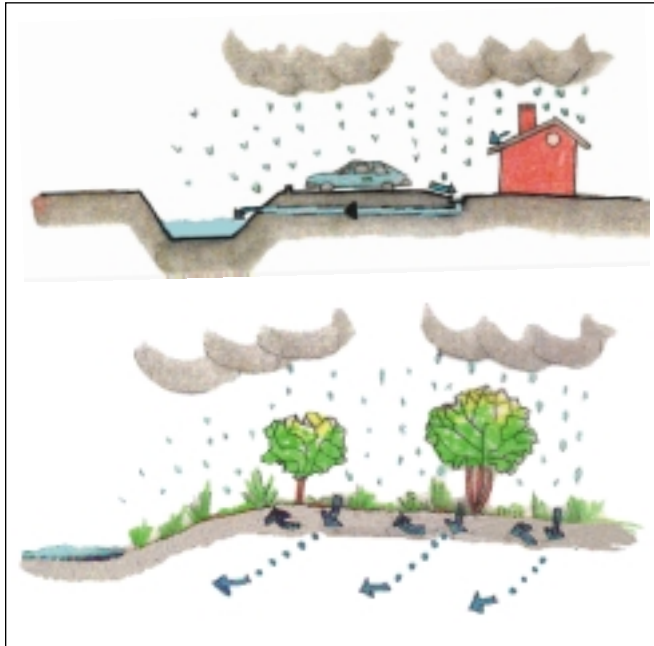
Urban impervious cover generates excessive runoff during storms, which is conventionally routed into pipes or concrete channels, robbing the soil of moisture and bypassing its absorptive capacity. In contrast, rain infiltrates into vegetated soil, recharging ground water and supporting plants. Drawing by Jen Uncapher, RMI.
