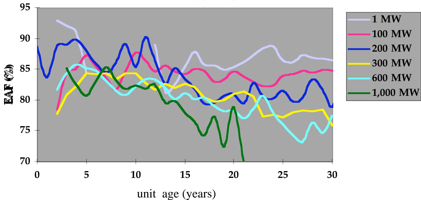
Fossil-fueled steam units: median Equivalent Availability Factor vs. age, by size range, 1982-93
