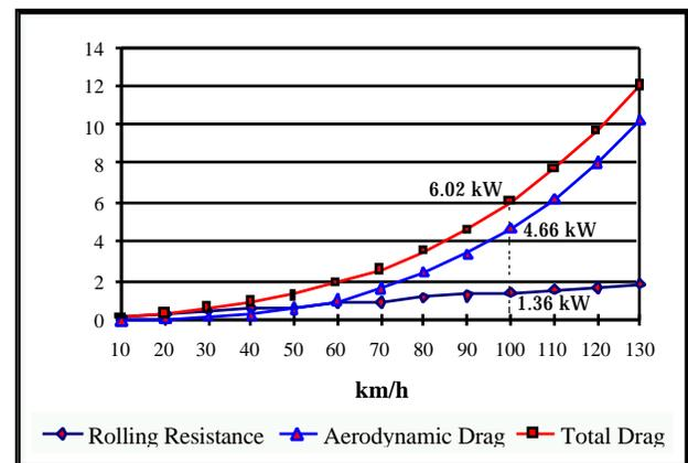
Figure 2 Reduced tractive loads on level ground
