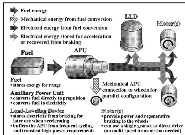
Figure 1 Series and dual-mode-parallel HEV schematic
