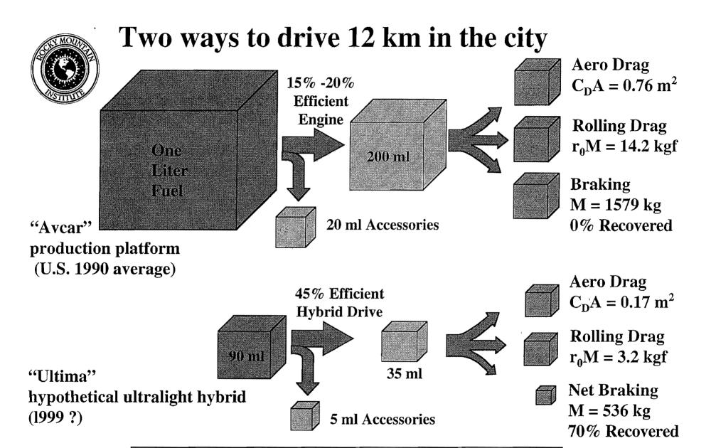
In highway driving, efficiency *falls* because there is far more irrecoverable loss to air drag (which rises as v<sup>3</sup>) and less recoverable loss to braking.
