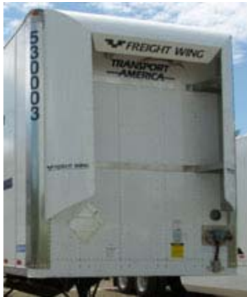
Gap Fairing, nose cones save ~2%
