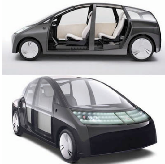
Figure 1. Toyota's impressive 1/X carbon-fiber concept car (2007) has the interior space of a Prius midsize hybrid, but is three times lighter and twice as fuel-efficient. Its half-liter flex-fuel engine, tucked under the rear seat, is supplemented by grid electricity via 20 extra kg of batteries. The plug-in hybrid's remaining curb
