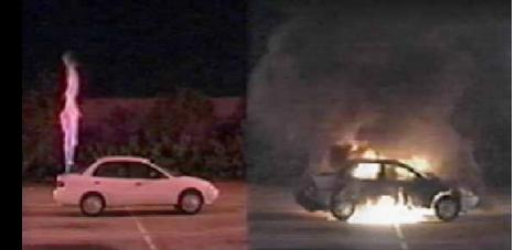
60 s:  $H_2$  flow subsiding; max 47°C on rear window, 19.4°C on tray behind rear seat. Zooming in on gasoline car...
