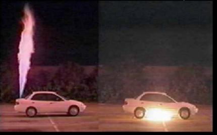
3 s: Ignition. H<sub>2</sub> @ 28 L/min, gasoline @ 0.68 L/min
