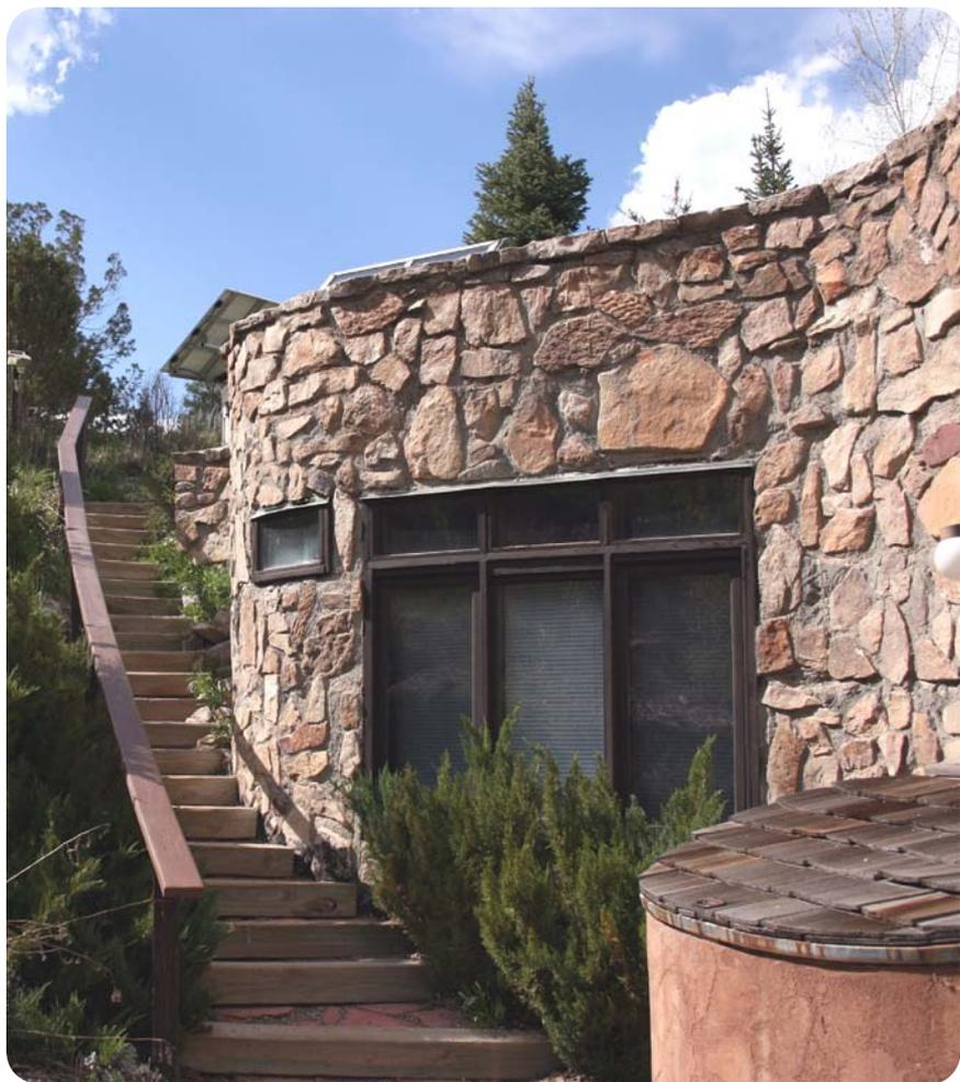
**West Bedroom:** The bedroom wing, being far from the greenhouse (the “furnace” of the building), is heated by its south- and southeast-facing windows (plus surplus heat from the people, lights, and minor heat leakage from a superinsulated solar-hot-water storage tank), so it stays a few Fahrenheit degrees cooler than the main wing, yielding more comfortable sleeping conditions.
