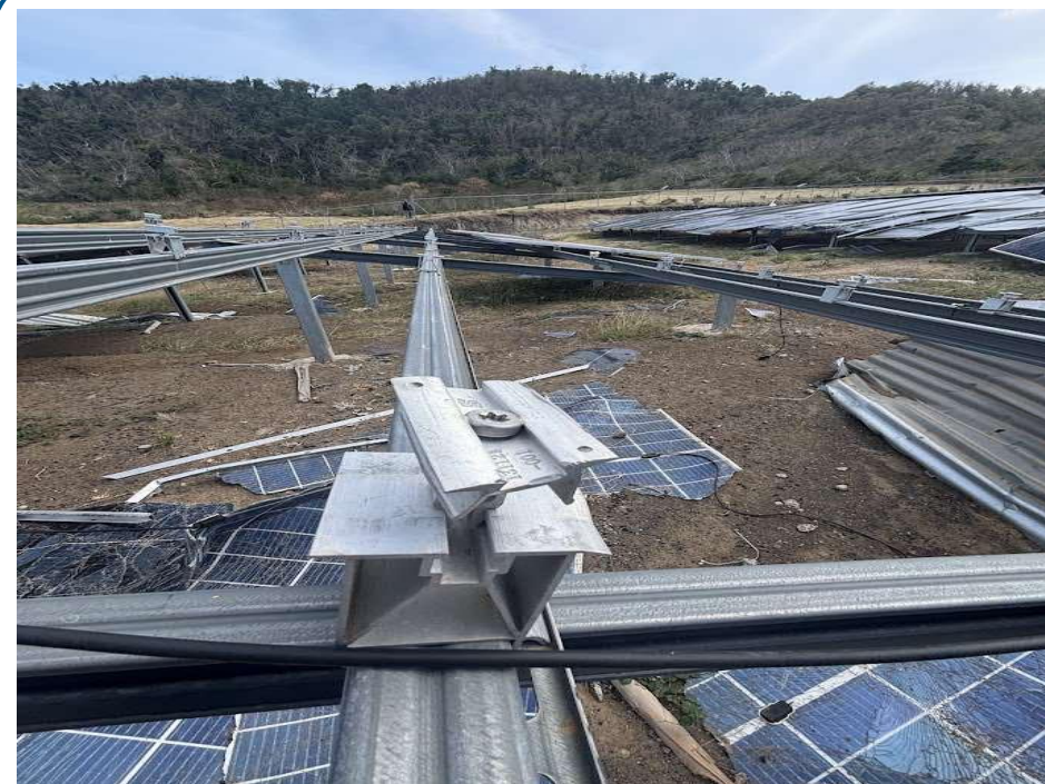
Cascading failure of T-slot risers and top-down clamps on Carriacou, Grenada during Hurricane Beryl.
