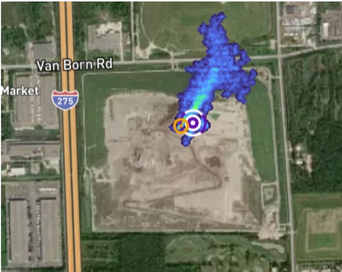
A methane plume detected at a Michigan landfill with an energy project. Methane Imagery © Carbon Mapper https://data.carbonmapper.org .
