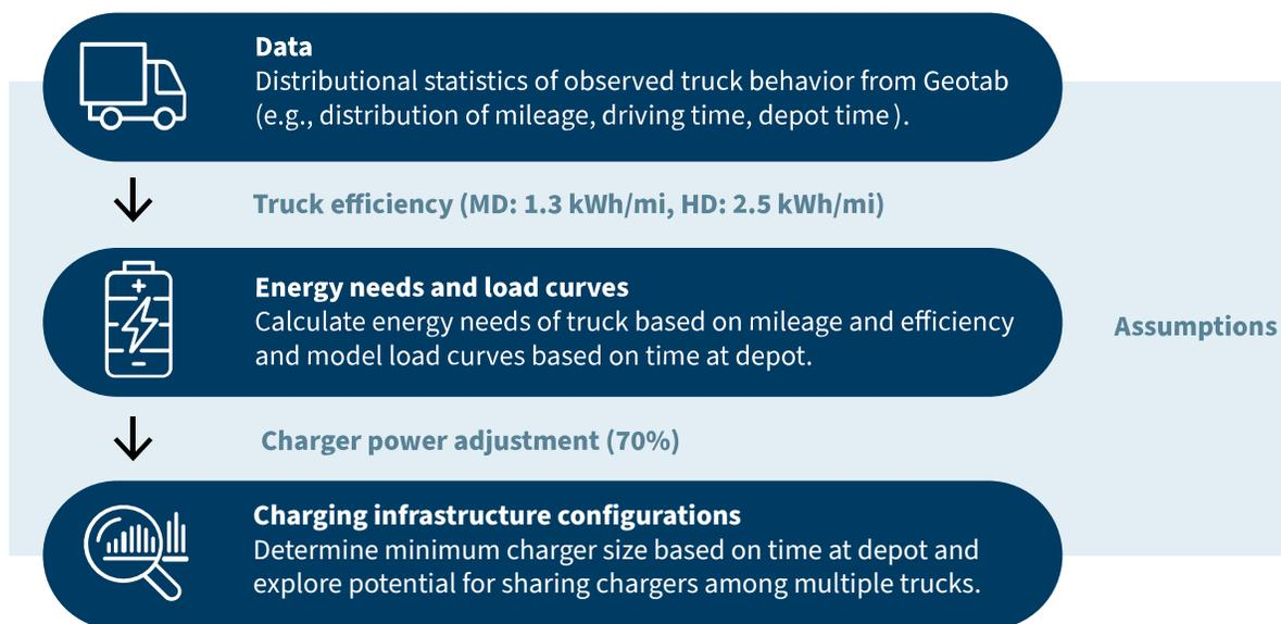
RMI Graphic. Source: Geotab ITS based on real-world truck telematics data
