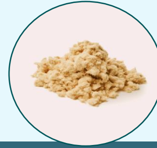
Blow-in fiber insulation
